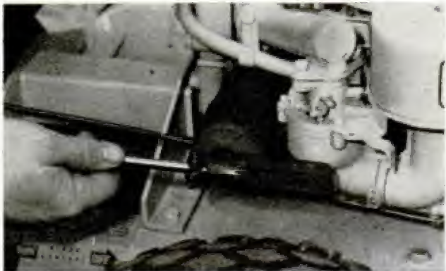
A STUCK NEEDLE VALVE can often be loosened by tapping on the carburetor bowl with a screwdriver
